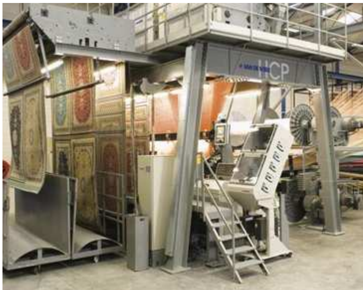
Figure 4: the three rapier Handlook Carpet Pioneer HCP X2 machine
