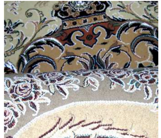
Figure 2: the handlook HCP X2 weave structure, woven with three rapiers, giving double production with no visible warp yarns at the back side of the carpet; pile and back side of HCP X2 carpet in reed 700 d/m
